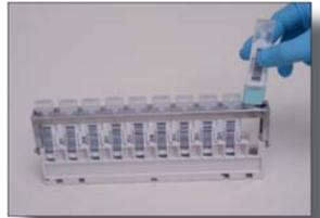
Sample is bar code labeled and placed on the OC-Auto Micro 80 iFOB sample rack
