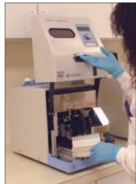
Sample rack is loaded into the OC-Auto Micro 80 iFOB analyzer
